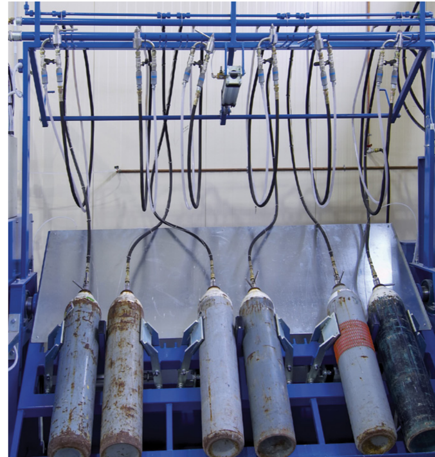
Hydraulic 6-Position Testing Machine for Gases & Cylinders Maximum Production Capacity of 30 Cylinders per Hour - Maximum Test Pressure 450bar
